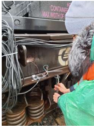
Figure 3.2 – Measurements of the parameters of the main bearing elements of the flat car
