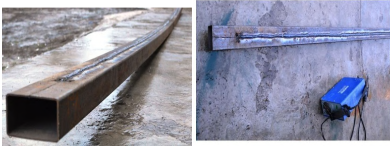
Fig. 3.2. Top cord test sample after technological welding
