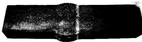
Fig. 3.15. Microslice for research into structural states of materials in zones of temperature impact at thermal straightening
