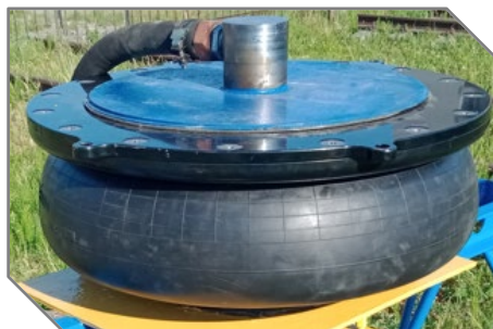
Figure 1. Pneumatic spring of high-speed rolling stock
