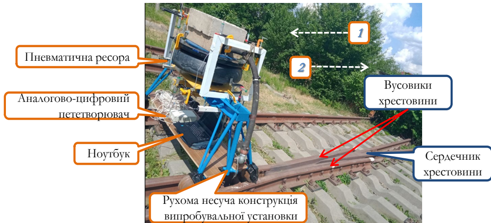
Figure 2. Installation for running dynamic tests of a pneumatic spring: 1 – Direction of movement from the core to the crosspiece moustache; 2 – Direction of movement from the crosspiece moustache to the crosspiece core
