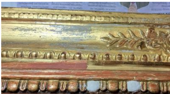
Figure 18. Scuffs on matte gilding areas on a large listel before tinting at the loss sites
