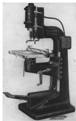
8. *Combination disk and spindle sander*, adaptable to the majority of sanding operations and is the type generally used in the wood shop.
