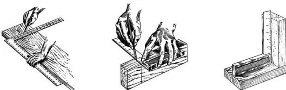
3. *Marking gage* was used for marking lines parallel to a surface of wood stock.
