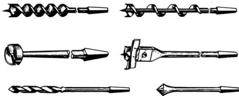
9. Drills: holes smaller than  $\frac{1}{4}$  inch are usually drilled with an automatic drill or small hand drill. These drills are faster and less cumbersome than the brace.
