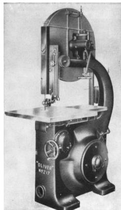
3. *Jig saw* differs radically in construction from the band scroll saw although the type of work for which it is intended is very similar. It is more adaptable for cutting small, sharp curves because much smaller and finer blades may be used.
