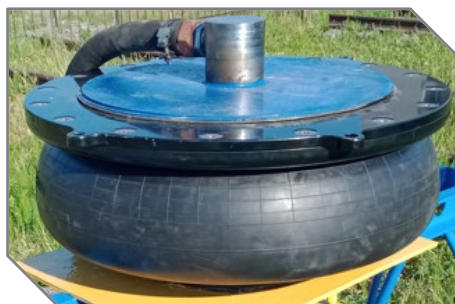
Figure 1. Pneumatic spring of high-speed rolling stock
