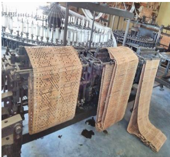
Figure 4. Lacemaking mechanism with punctured cards
