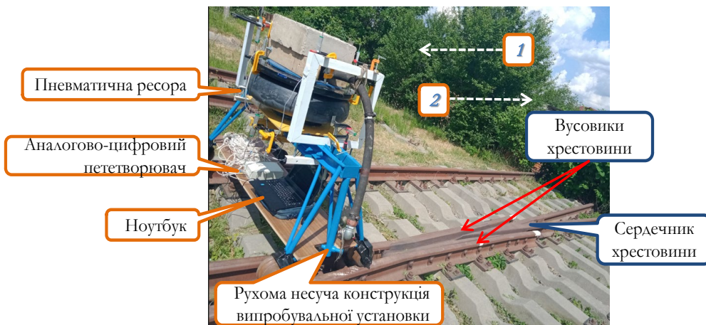
Figure 2. Installation for running dynamic tests of a pneumatic spring: 1 – Direction of movement from the core to the crosspiece moustache; 2 – Direction of movement from the crosspiece moustache to the crosspiece core
