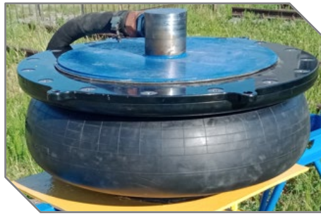
Figure 1. Pneumatic spring of high-speed rolling stock
