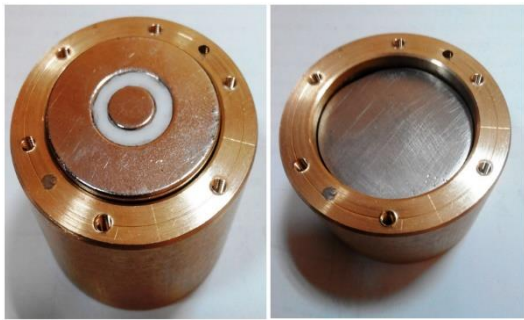
Figure 3. Photo of the developed magnetron
